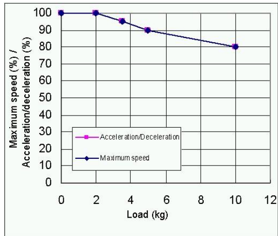
Setting of maximum speed and acceleration/deceleration in relation to load mass (Axis 4)
